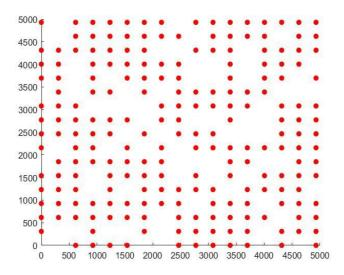
Figure 9: Optimal Placement of Wind Turbines Using Genetic Algorithm with Static Values of Crossover and Mutation Factors for Layout of Dimension 5000 m x 5000 m
